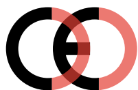
False CE Mark (too close)
