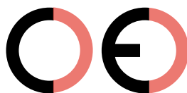
False CE Mark (too far)
